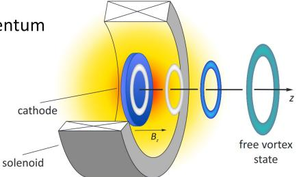
Electrons emitted with L = 0 on the cathode carry the canonical angular momentum,
